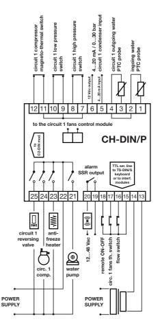
This alarm disables the compressor and the fans, turns the "Alarm" led on and enables output SSR 12...48 Vac.
